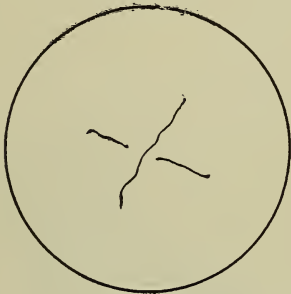
Fig. 2.—Soundness Pat Showing Shrinkage Cracks
